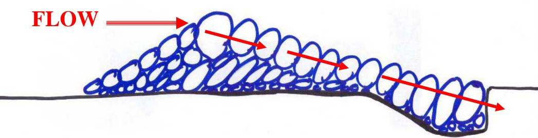
Weighted toe can designed to help stop the headward migration of a DS knickpoint {headcut}
