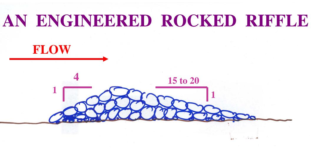
Largest stones are placed at crest and on downstream face, upstream face is in compression due to water flow
