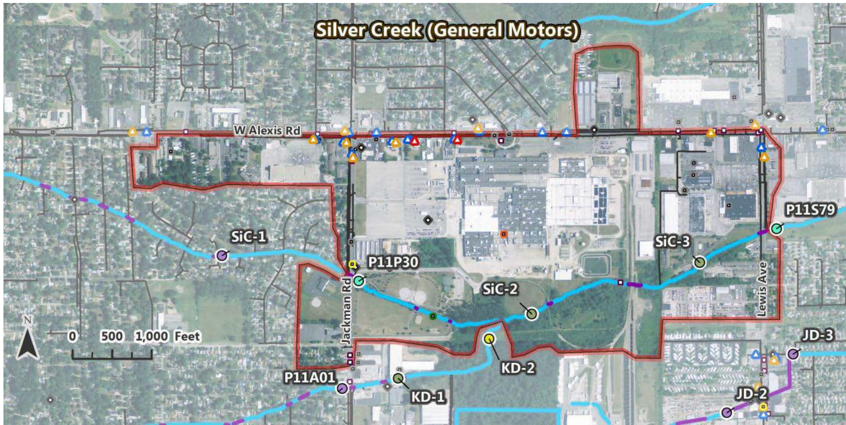
Figure 27. Recommended sampling locations along Silver Creek upstream of and in the General Motors critical area.
