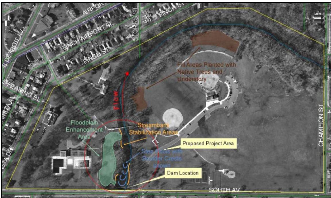
*Initial conceptual design with step pool drop structures.*
