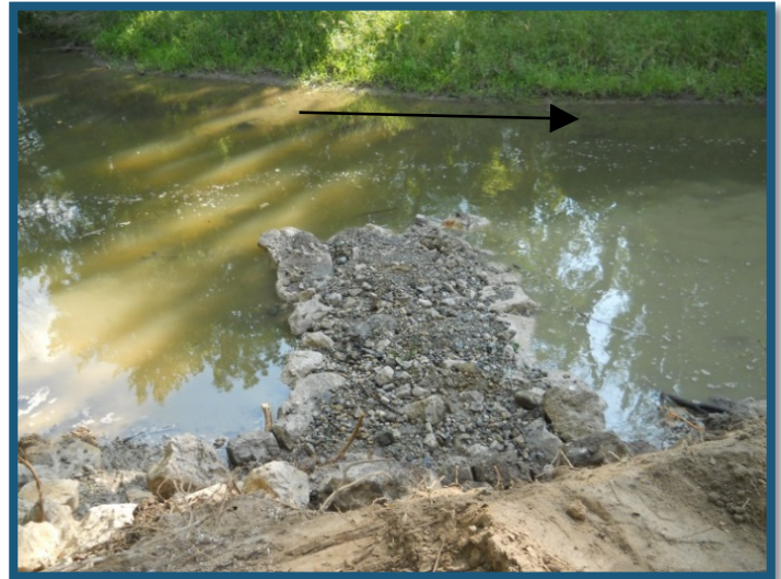
Image 2: Bendway Weir and thalweg (bubble line) at Camp Miakonda in Sylvania, OH. Kyle Spicer
